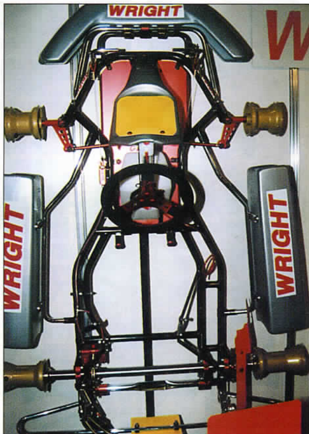
This is the Garda 03, the 02 model looks identical but is wider front and rear
