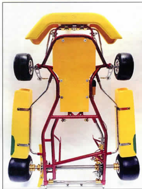
The Taurus has an additional cross-member linking the steering yokes
