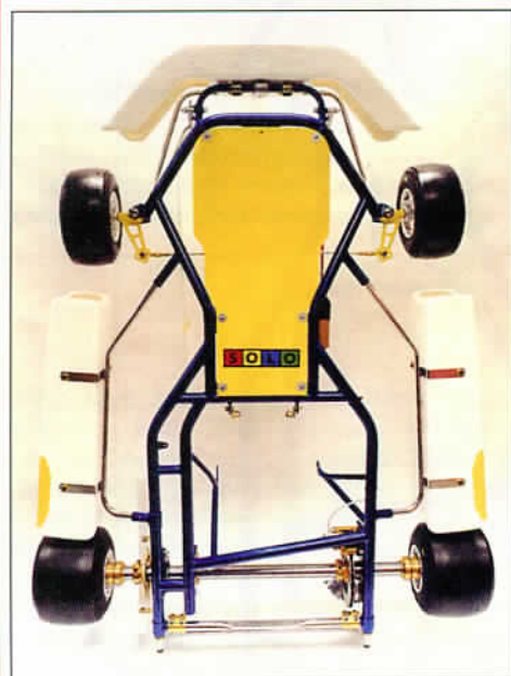
The Tornado's waist section side rails join the front and middle cross-members
