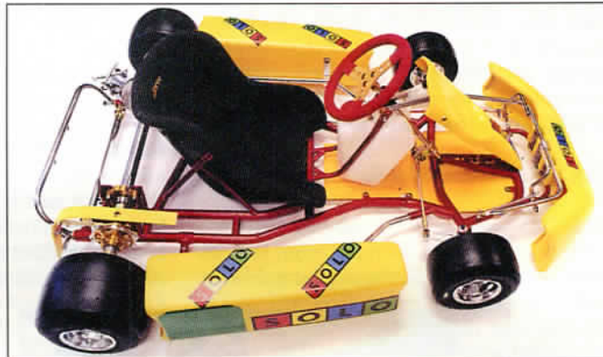
The Taurus has an additional cross-member linking the steering yokes
