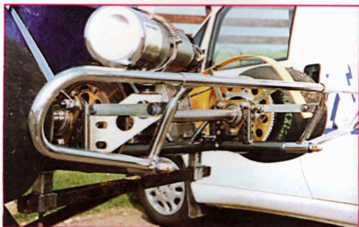
Well made rear bumper on the Spirit with sleeves over the main tube to prevent breakages
