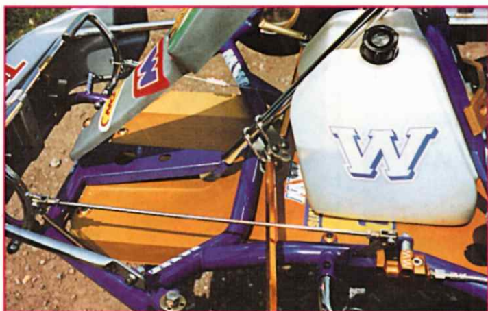
The Mike has a permanent cross member between the stub axles and a multi-position steering column
