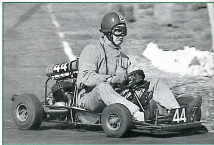
Comet 'JM' special with John at the wheel. Power was provided by twin Montesa 100 engines driving through a Manx Norton clutch fitted on the rear axle and hand operated
