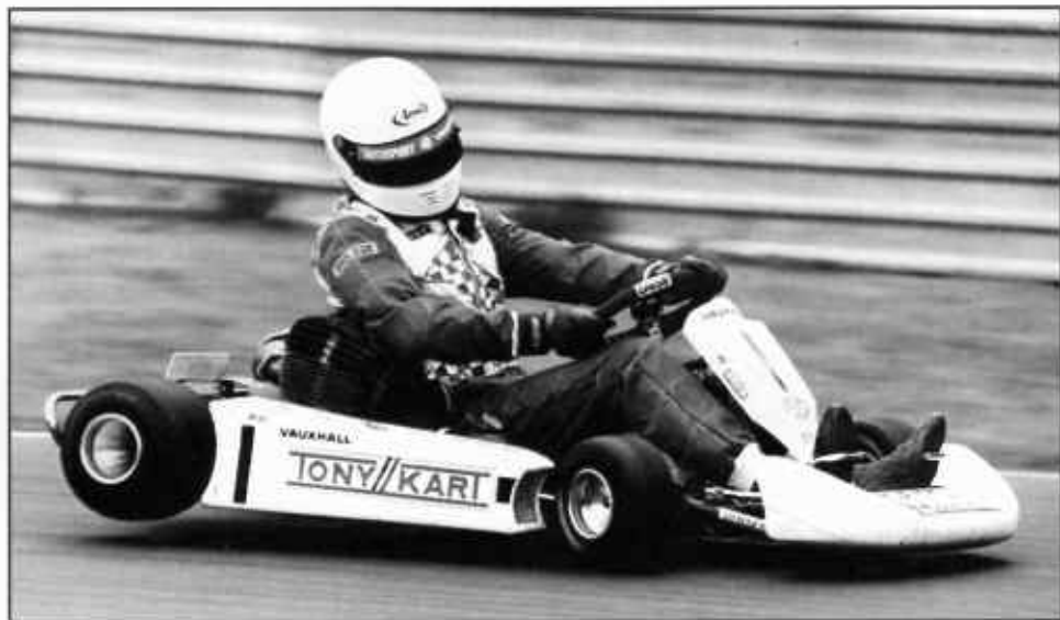
Figure 1. Kart decelerating and turning into a corner. As the weight transfers to the front left wheel it causes the front left corner to flex upwards. Since the chassis is rigid, the diagonally opposite wheel lifts
