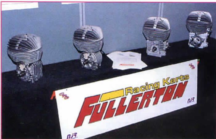
Note the new crankcase shape of the new CRGs compared to the S20 (second from the left)
