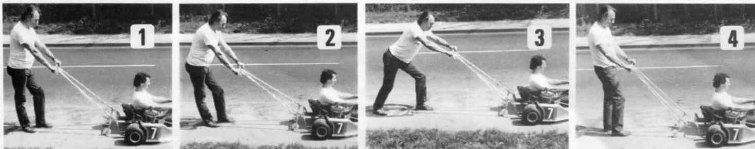
1. Hook onto the rear bumper. 2. Lower handle to raise kart wheels off ground. 3. Push kart. 4. Press trigger, kart drops to ground, pushing continues until kart accelerates away.
