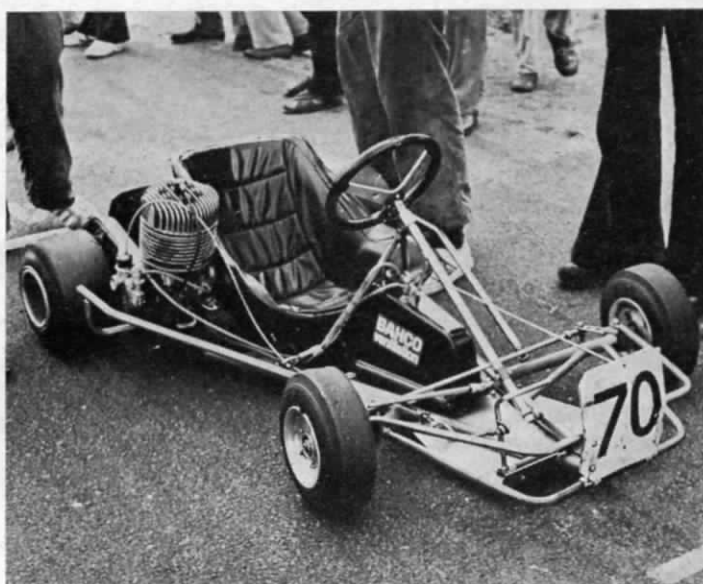
The leader on points after the heats, Sweden's Leif Larsson, was driving this B.M. powered Myhrman. The side nerf bars were coupled to the front axle by a ball joint so they did not affect frame flexibility.
